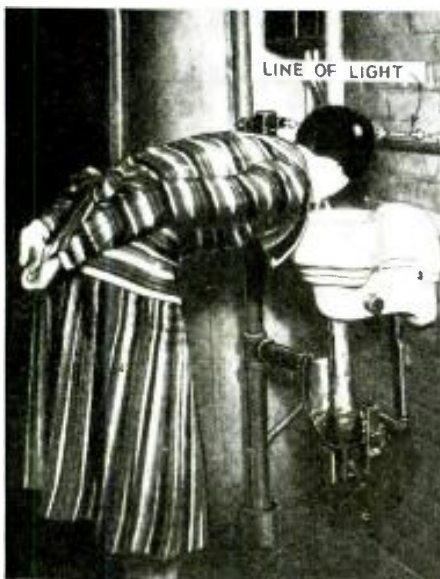
Fig. E PE. cell provides automatic drinking service.
