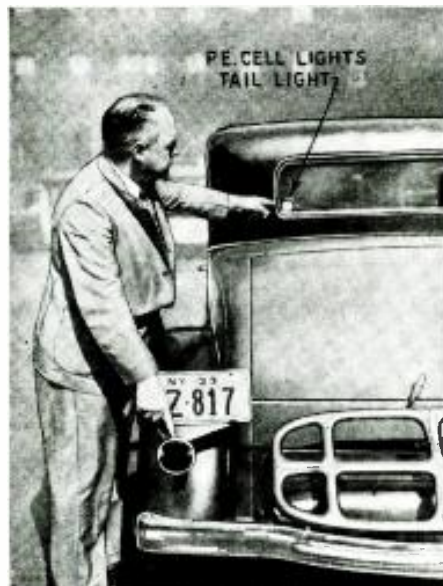
Fig. G.—PE cell turns on parking light.
